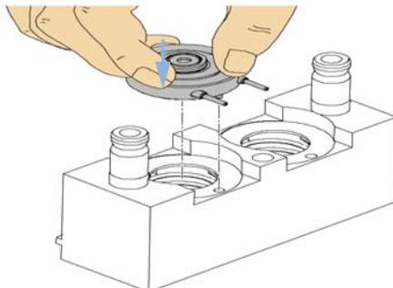
**Figure 22** Inserting the active seal wash support rings.
