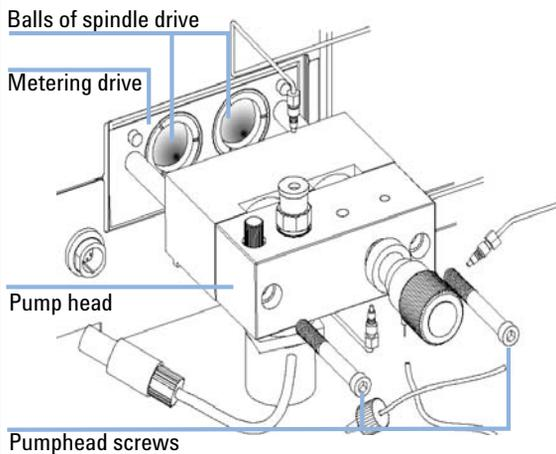
**10** Reconnect all capillaries, tubes and the active inlet valve cable to its connector.
