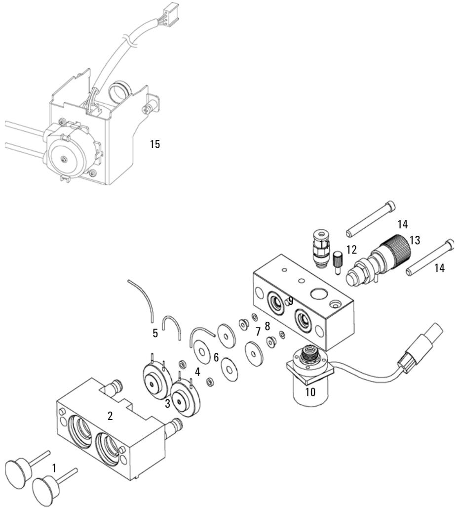
**Figure 28** Pump Head with Seal Wash Option
