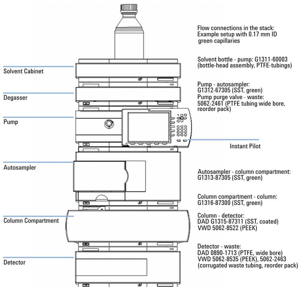
**Figure 5** Recommended Stack Configuration (Front View).
