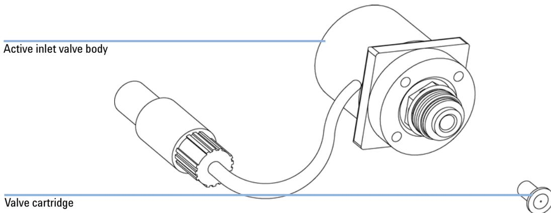
**Figure 14** Active Inlet Valve Assembly
