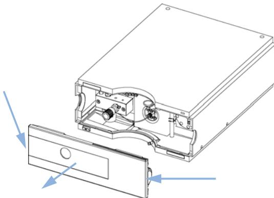
**Figure 9** Removing the Front Cover
