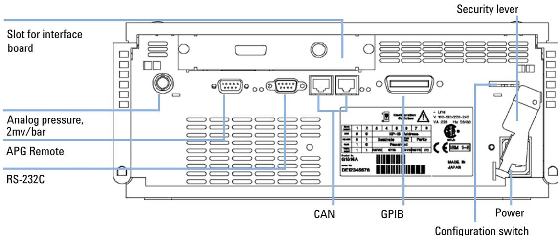
Figure 8 Electrical Connections
