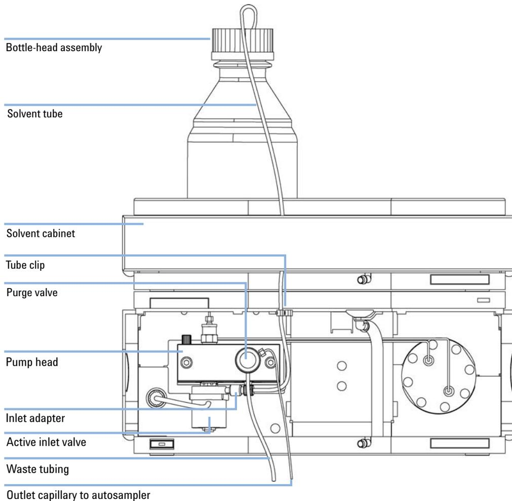
**Figure 10** Flow Connections of the Isocratic Pump
