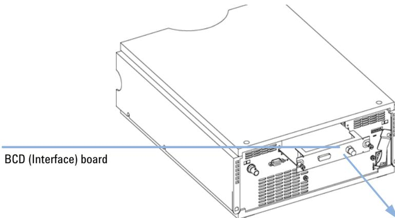
**Figure 24** Exchanging the Interface Board
