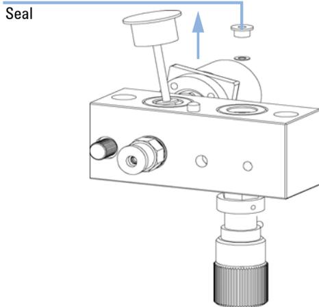
**4** Insert new seals into the pump head.
