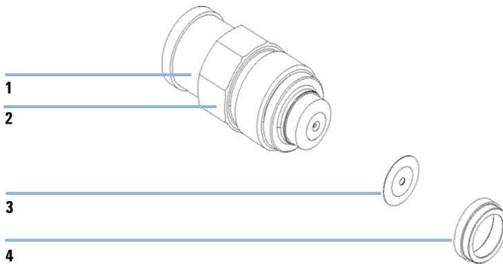
**Figure 29** Outlet Ball Valve Assembly
