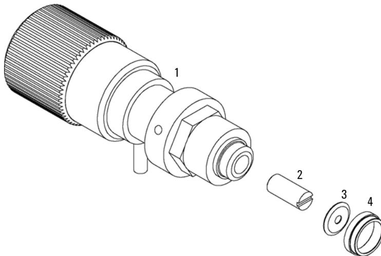
**Figure 30** Purge-Valve Assembly
