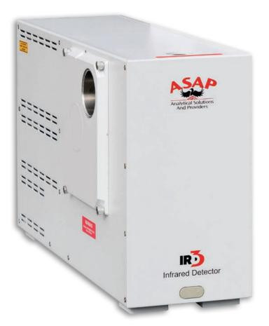
The IRD 3 is the perfect tool for the chromatographer looking to obtain more information about unknown samples that would not be possible with a MS detector. Using a heated light pipe flow cell, the sample is kept in the vapor phase while interacting within the IR band width. This allows the molecules to freely rotate in a low energy environment. Keeping the molecular geometry intact during analysis provides a unique and highly reproducible spectra.
