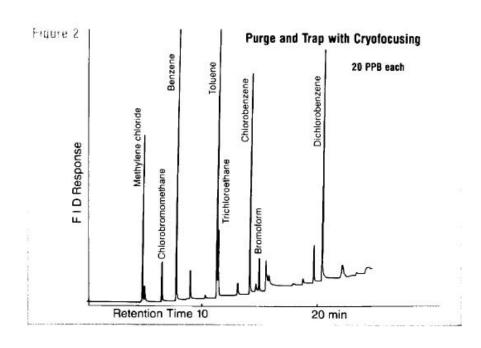
Automatic cryofocusing improves the sensitivity by eliminating the need to split the sample at the injection port when using narrowbore capillaries, and thereby permits operation in the low PPB to parts-per-trillion range. Figure 2 is a chromatogram of a variety of purgables present in a 5ml water sample at 20PPB, using a 0.75mm capillary column. The use of a 0.25mm column with cryofocusing has permitted the determination of aromatics at a concentration of less than 10 parts-per trillion.
