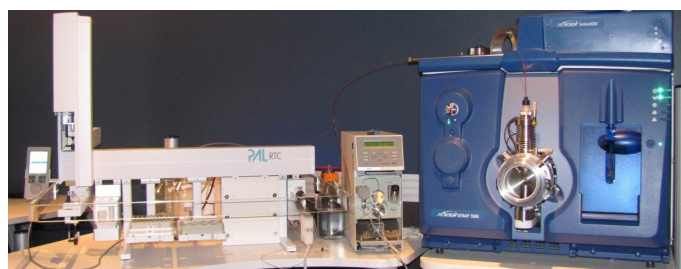
Fig. 1: RTC system and a LC coupled to a MS/MS Sciex QTRAP ® 5500 System in MRM mode
