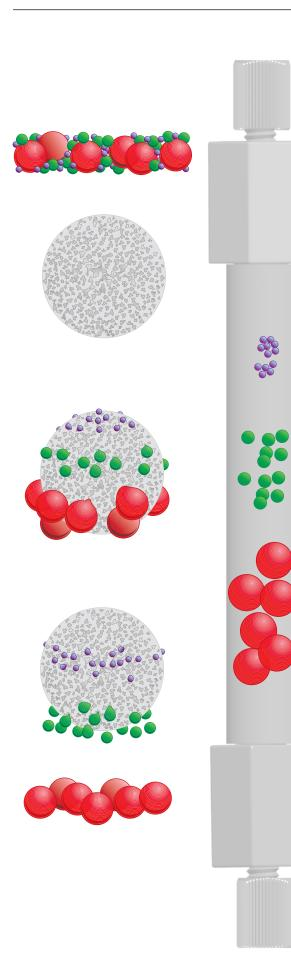
Size exclusion chromatography (SEC) is a method in which components of a mixture are separated according to their molecular size, based on the flow of the sample through a porous packing. In contrast to all other modes of liquid chromatography the prerequisite for SEC is that the analyte does not interact with the surface of the stationary phases. Differences in elution time are ideally based solely on the volume the analyte passes.
